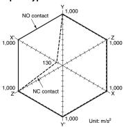
Sample: G2RL-14 12 VDC Number of relays: 5 pcs Test conditions: Shock is applied
