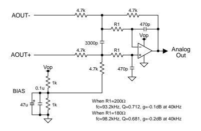
Figure 11. External 2<sup>nd</sup> order LPF Circuit Example (using op-amp with single power supply)
