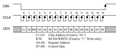
Figure 9. Control I/F Timing
