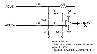
Figure 12. External 2<sup>nd</sup> order LPF Circuit Example (using op-amp with dual power supplies)
